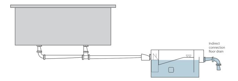
Drawing shows a code compliant indirect sewer connection.
